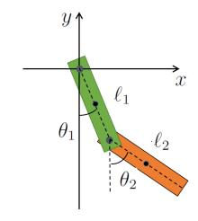
First, we derive the Lagrangian L. Suppose that the co-ordinates of COM of each arm be  $(x_1, y_1)$  and  $(x_2, y_2)$ , then they can be expressed in terms of the angles  $(\theta_1, \theta_2)$  as
